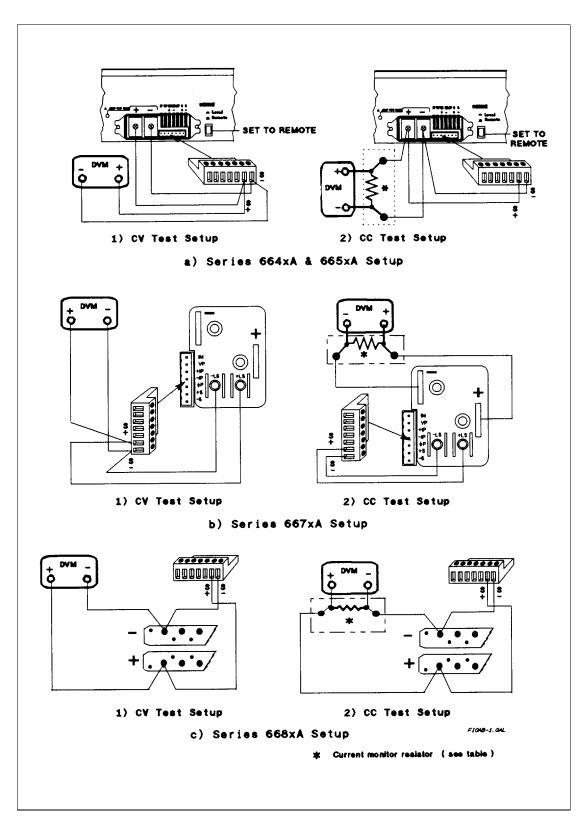
Figure A-1. Calibration Test Setup
